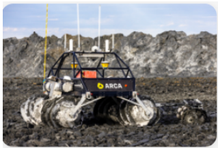
Arca rover conducting Smart Churning on mine tailings
