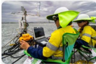
Arca scientists monitoring carbon flux into mine waste
